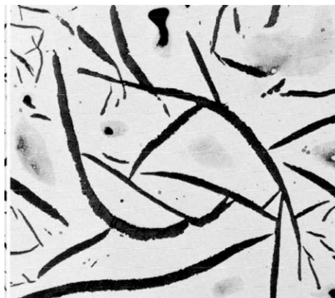
Figure 7.18. Microstructure of gray cast iron. The black flakes are graphite. The white areas are ferrite and the gray areas are pearlite. From American Society for Metals, Metals Handbook , 8th ed., v. 8, 1982.
