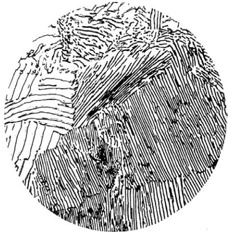
Figure 7.2. Microstructure of pearlite. Note the alternating platelets of ferrite (white) and iron carbide (dark). From Making, Shaping and Treating Steels , 9th ed., United States Steel Corp., 1971.
